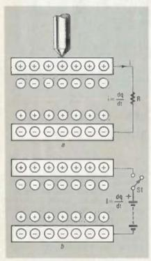
FIG. 1—A CAPACITOR CAN BE CHARGED by a gravitational impulse (#), just as it may by a DC voltage (b).
