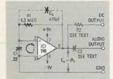
FIG. 2—A BASIC GRAVITY-WAVE DETECTOR Is very simple. The charge build-up on capacitor CI due to gravity-wave impulses is amplified by ICI for output.
